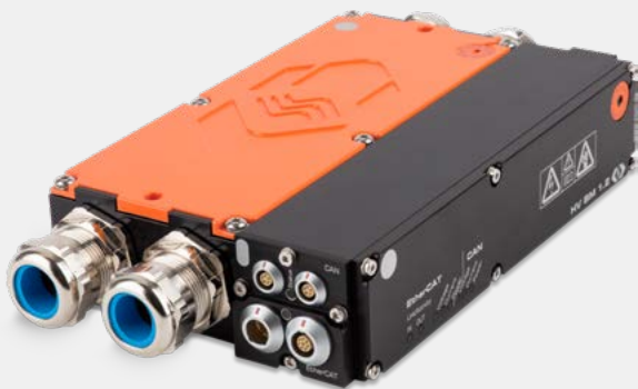
Fig. 4: HV Breakout Module 1.2 for measuring current, voltage and power in the separate HV+ and HV- lines between fuel cell stack and DC/DC converter.
