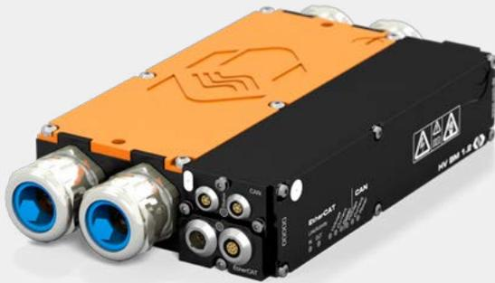
Fig. 4: HV Breakout Module 1.2 for measuring current, voltage and power in the separate HV+ and HV- lines between fuel cell stack and DC/DC converter.
