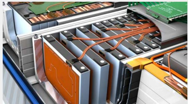
Fig. 6: IC sensors on ultra-thin flexible circuits are suitable for precise temperature measurement between the battery cells.
