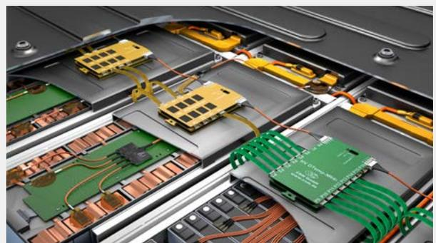
Fig. 7: HV DTemp-M64 Controller for the connection of up to 64 IC sensors.
