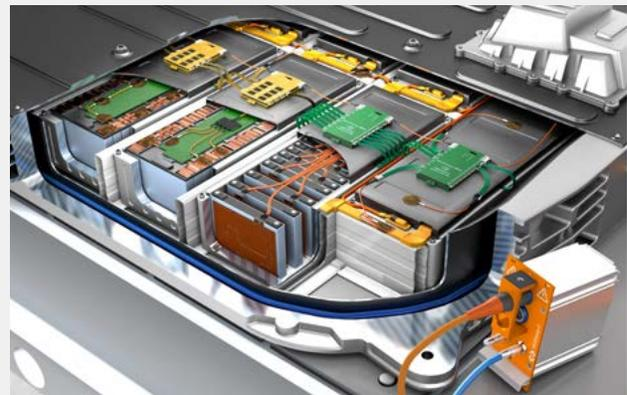
Fig. 1: HV DTemp measurement system installed in a HV battery
