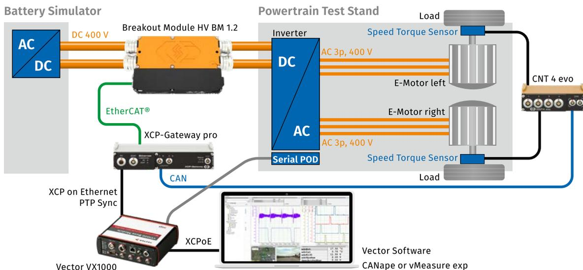
Fig. 4: Vector CSM E-Mobility Measurement System for efficiency analysis of a powertrain. The eMobilityAnalyzer for power analysis is an integral part of Vector CANape and vMeasure exp software.
