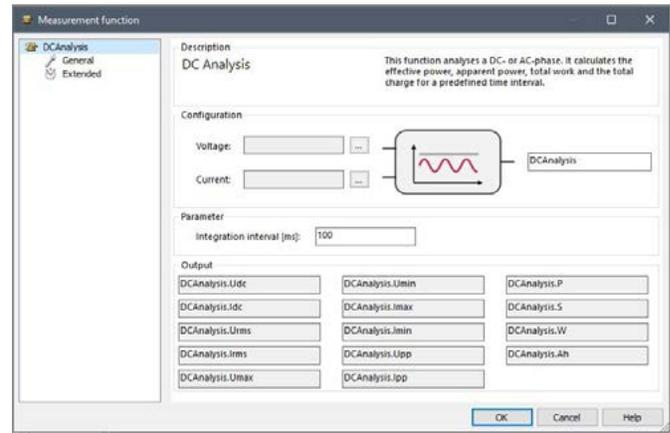
Fig. 5: The DC Analysis function for power analysis on a DC line. The input variables are the sampling values of voltage and current from the HV BM 1.2. The effective power, apparent power, total work, and total load are calculated from a predetermined equation.
