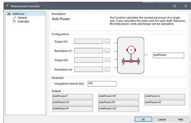
Fig. 1: The Axle Power function calculates the mechanical performance and total power from the signals of the speed torque sensors on the each of the two axles
