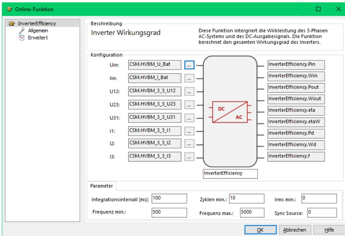
Fig. 4: Efficiency analysis with the eMobilityAnalyzer
