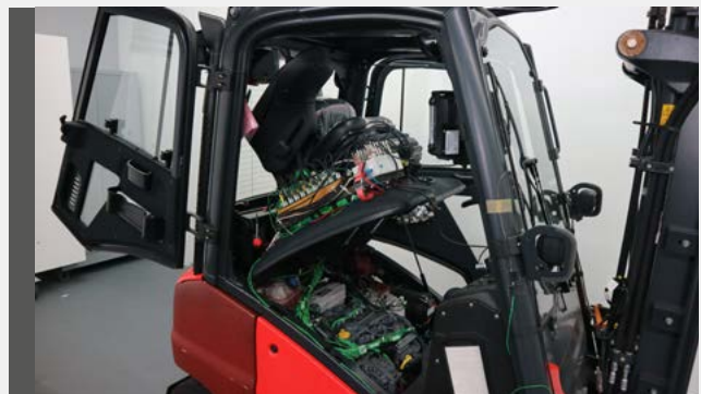
Fig. 4: This image shows the compact measurement modules in the cabin, located directly above the instrumented engine compartment.
