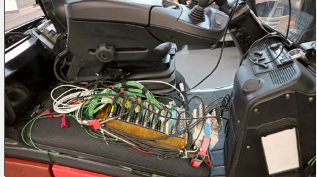
Fig. 3: With CSM's unique Slide Cases, all of the measurement modules are locked together to make a compact hardware system in the cabin.
