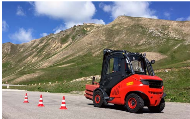
Fig. 1: In the high altitude test, a forklift truck is tested at 2,400 m in the Alps. After engine integration, the vehicle must function perfectly and still meets regulatory requirements.
