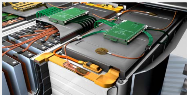
Fig. 4: HV DTemp IC single sensors on the module housing and busbar.
