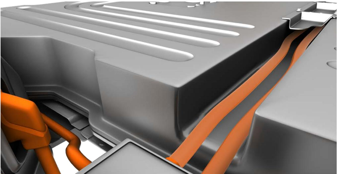
Fig. 6: Narrow cable ducts offer only limited installation space for the measurement technology to measure current and voltage in the HV power cables.
