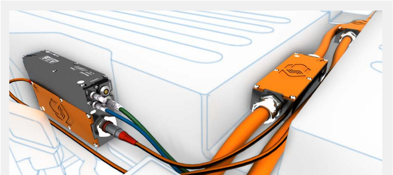
Fig. 8: High-voltage current and voltage measurement in a narrow cable duct. The Split Breakout Modules (HV SBM\_I, HV SBM\_U) for current and voltage are connected with high voltage safe sensor cables to the Split Acquisition Module (SAM). This is connected to the measuring computer via CAN or EtherCAT®.
