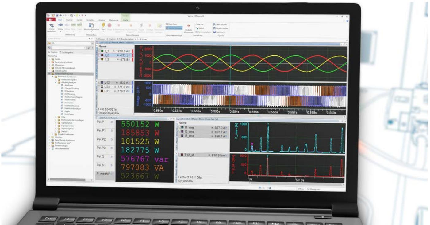
Fig. 4: Performance analysis of a ten-minute test run on the test bench with CANape. The raw values of the phase-to-phase voltages and string currents are shown in the upper area. The electrical values calculated in the process, such as active, reactive and apparent power, and the calculated mechanical power are listed numerically at the bottom left. The three calculated effective values of the motor currents are shown at the bottom right.
