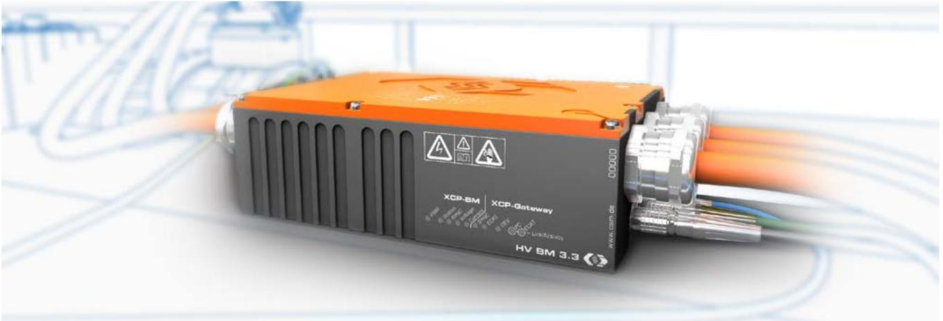
Fig. 6: HV Breakout Module 3.3.: The measurement system can be extended with further measurement modules via an EtherCAT and CAN interface. Via a Gbit Ethernet interface the data are sent to the measuring computer. Via the cable glands (shielded) HV cables up to 95 mm<sup>2</sup> are connected inside the housing.
