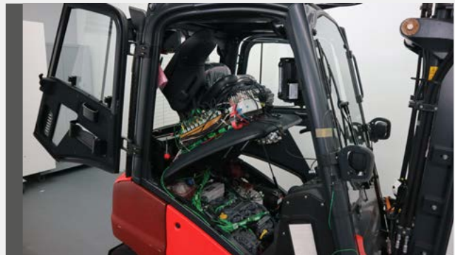
Fig. 4: This image shows the compact measurement modules in the cabin, located directly above the instrumented engine compartment.
