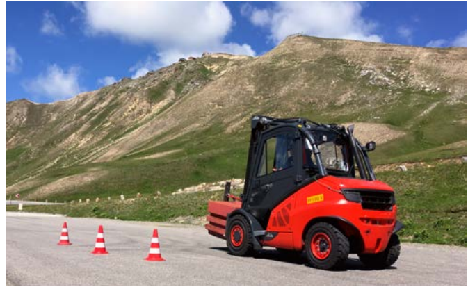
Fig. 1: In the high altitude test, a forklift truck is tested at 2,400 m in the Alps. After engine integration, the vehicle must function perfectly and still meets regulatory requirements.
