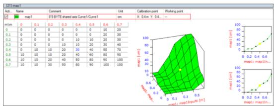
Numerical and graphical adjustment window allows convenient adjustment of characteristic curves and fields
