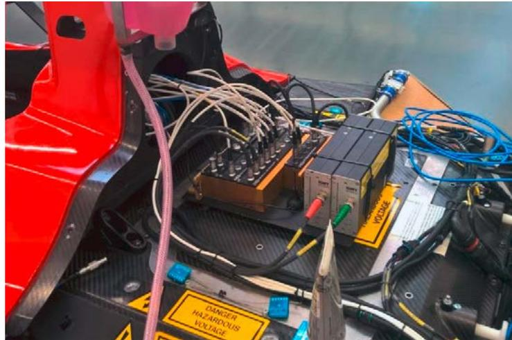
CSM MiniModules mounted for test operation
