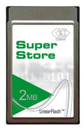
CSM PCMCIA Linear Flash Card AMD-C Series compatible conforms to PCMCIA/JEIDA international standard and consists of multiple AMD's or FUJITSU's or compatible 5 V Flash memory devices and decoder IC mounted on a very thin printed circuit board using surface mounting technology.
