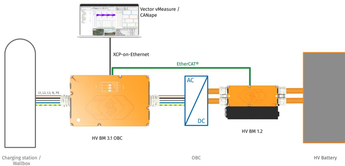
Fig. 2: Schematic measurement setup for current, voltage and power measurement between AC charging station and OBC in the vehicle.
