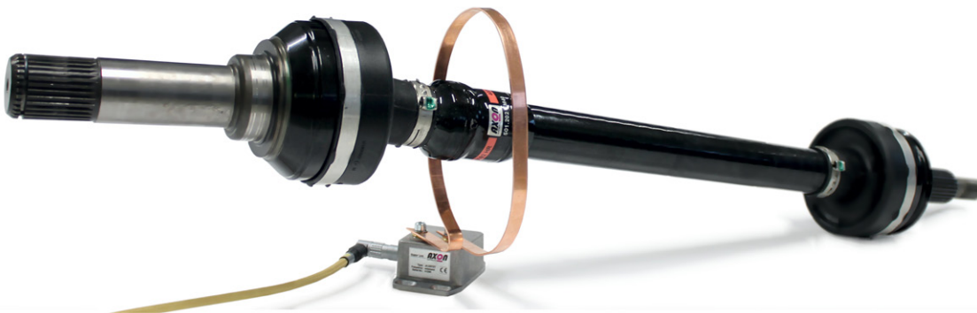
Fig. 2: AXON rotor electronics and antenna for non-contact transmission of the recorded data from the strain gauge and temperature sensor on the axle. (Photo: AXON Systems GmbH)
