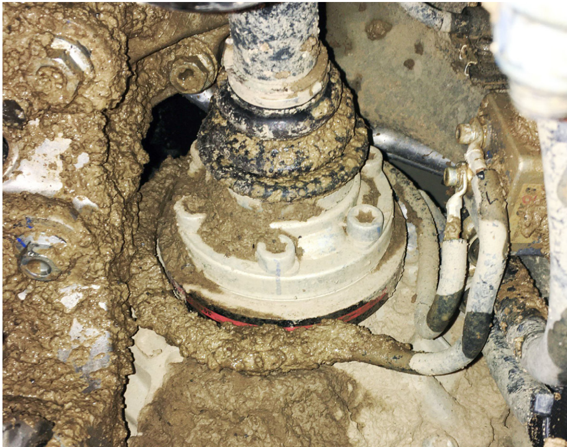
Fig. 4: In addition to sensors installed on the axle, AXON also offers torque measurement flanges for acquiring acting forces. The entire measurement technology is also suitable for harsh environmental conditions, such as off-road driving tests. (Photo: AXON Systems GmbH)
