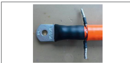
Fig. 5-43: HV BM 1.2+S, power cable HV+, strands of the braided shield, twisted, insulated and tinned
