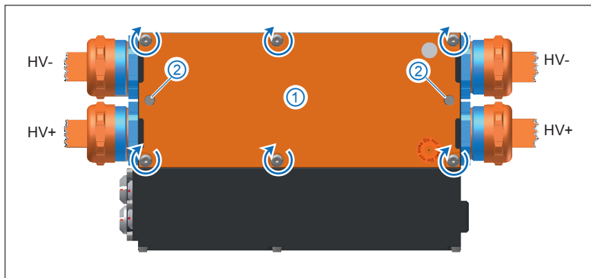
Fig. 5-18: HV BM 1.2, HV power cables mounted, housing closed
