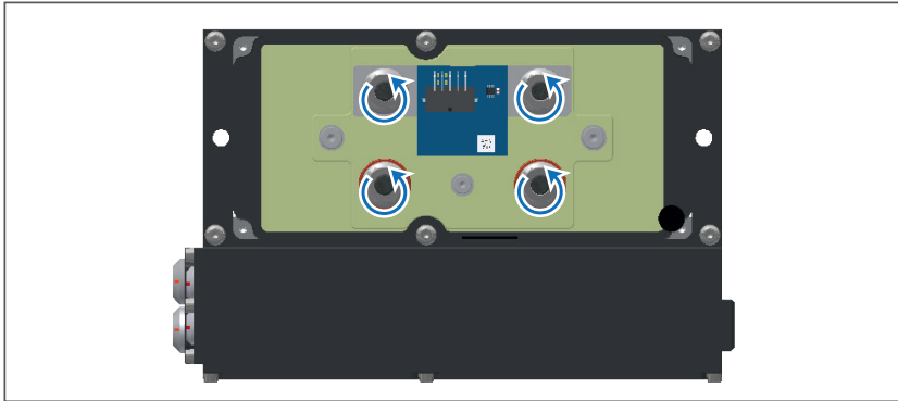
Fig. 5-3: HV BM 1.2, housing opened, loosen and remove the M8 nuts
