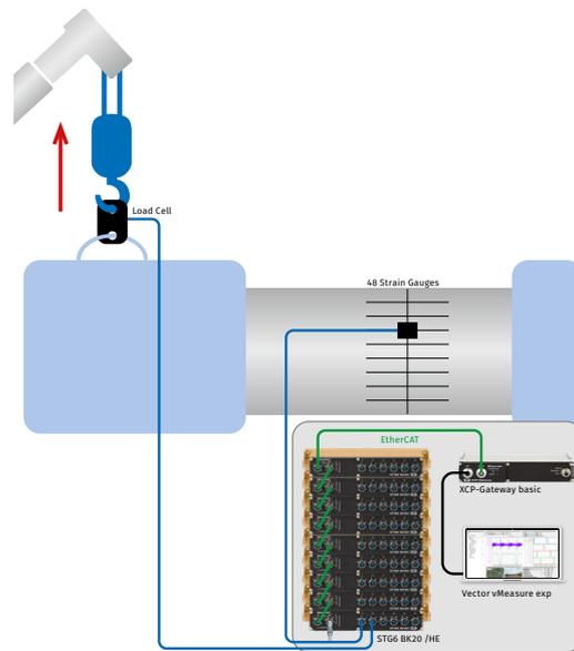
Fig. 2: The measurement modules are transported to the test area with the test specimen. Here, the test specimen is fixed on one side and the desired load is applied by lifting on the other end.
