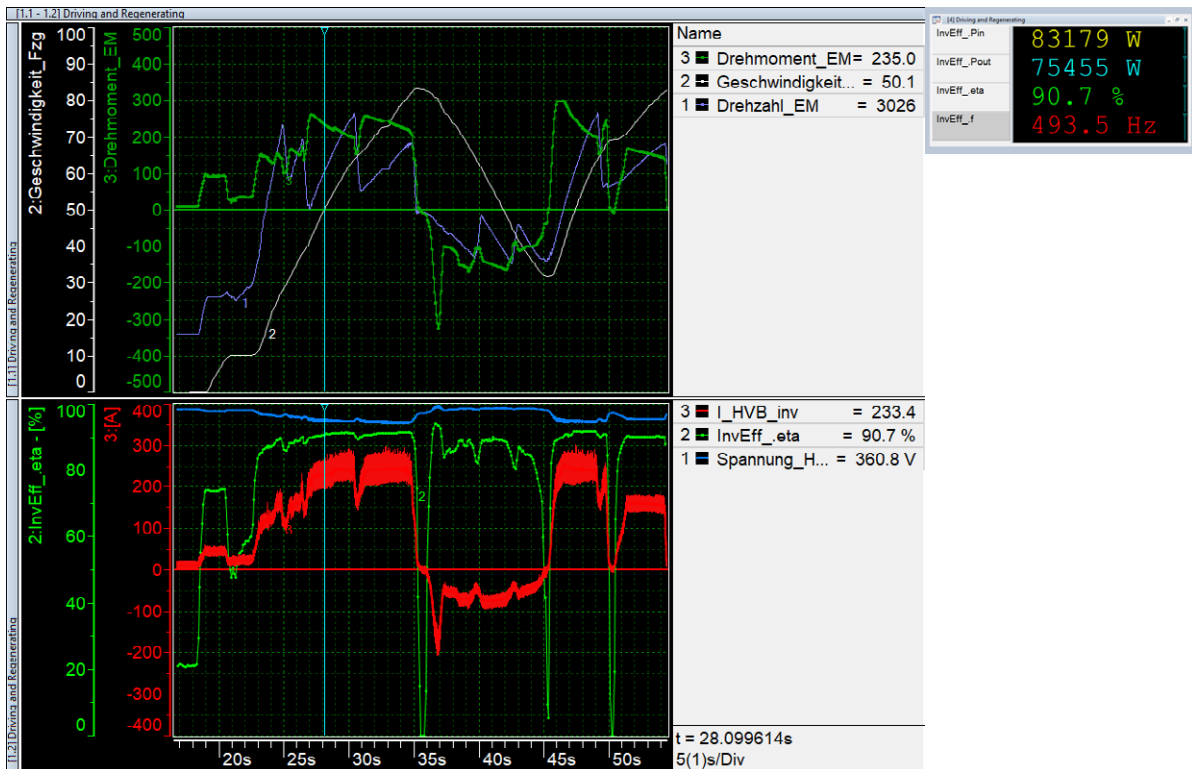
Fig. 6: Detail of a test drive of an electric vehicle with a nominal electric power of 75 kW and instrumented CSM Vector E-Mobility Measurement System (see Fig. 1). From the velocity profile shown in the upper plot (white), one can see when the vehicle accelerates and when it decelerates. Accordingly, the current shown in red in the lower plot is positive or negative. The vehicle's power electronics work as an inverter when driving, with efficiencies of over 90% at higher loads, and as a charger when the engine is operated as a generator during recuperation. When charging, efficiencies of up to 90% are also achieved. It can be seen that at small currents during load changes, the efficiencies of both the inverter and charger become worse. The calculation of the efficiencies can be done directly during the measurement or afterwards. It is done with the evaluation function (see Fig. 4) included in Vector's eMobilityAnalyzer function package (included in CANape and vMeasure). This evaluation function also determines the frequency of the motor currents, the rotating field.
