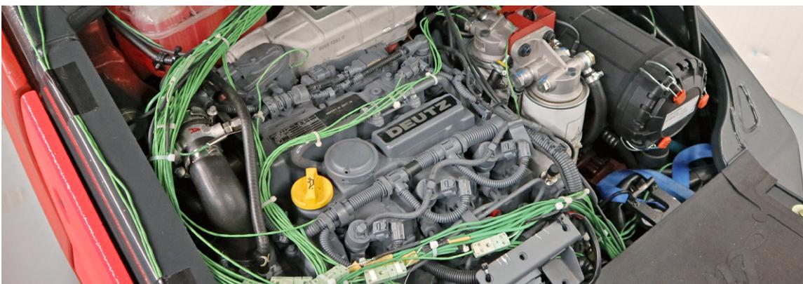
Fig. 3: The temperature and pressure sensors are installed in the specified locations in the engine compartment. The green cabling shows routing of the Type K thermocouple sensors to the measurement modules located outside the confined engine compartment.
