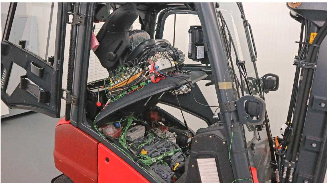
Fig. 5: This image shows the compact measurement modules in the cabin, located directly above the instrumented engine compartment.
