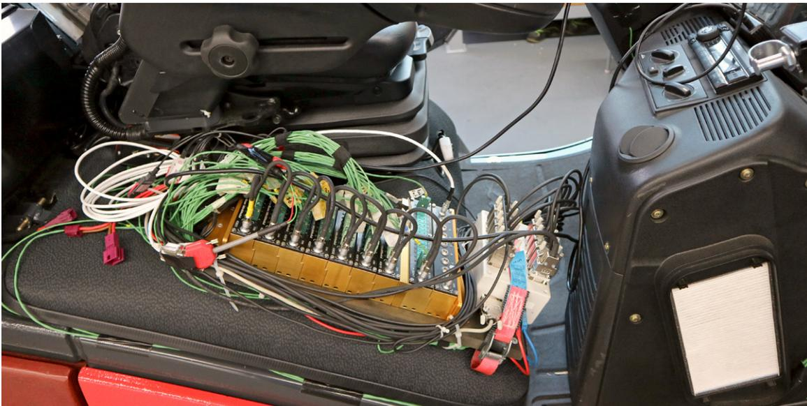
Fig. 4: With CSM's unique Slide Cases, all of the measurement modules are locked together to make a compact hardware system in the cabin.
