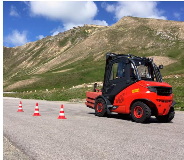
Fig. 1: In the high altitude test, a forklift truck is tested at 2,400 m in the Alps. After engine integration, the vehicle must function perfectly and still meets regulatory requirements.
