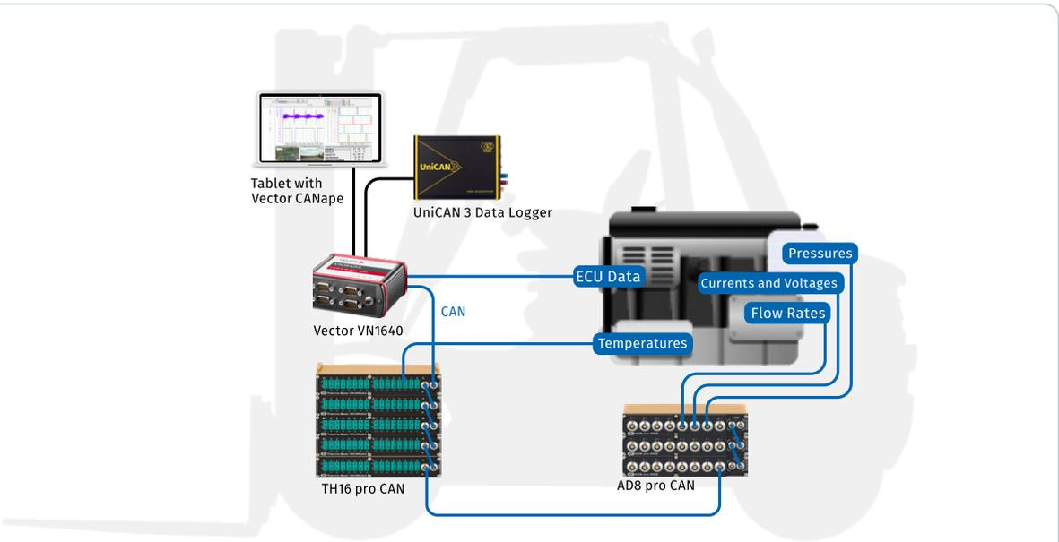
Fig. 2: THMM 16 pro Temperature measurement modules acquire the temperatures at different points in the engine compartment. Additional parameters are measured using AD8 pro MC2 modules. The measurement data is collected simultaneously with information from the ECU with the Vector interface VN1640, and is passed to a UniCAN3 data logger, as well as to a tablet for live display.
