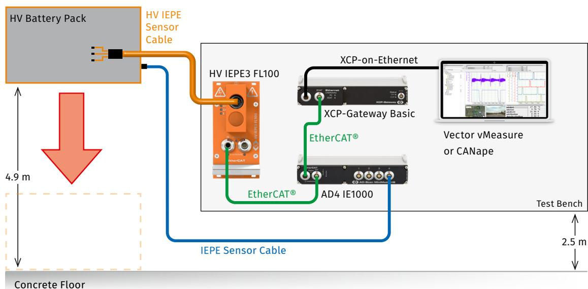
All measurement modules are placed at half the drop height to optimize the length of the signal cables and in order to minimize signal interferences.
