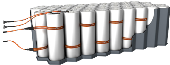
Fig. 9: IC sensors on ultra-thin flexible circuit as strips for temperature measurement between round cells.
