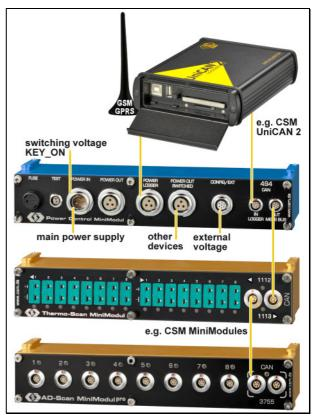
Figure 1: Example of a CSM measurement system with data logger.
