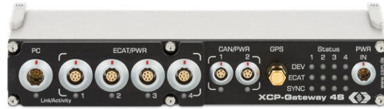
Fig. 2: An XCP Gateway 4S pro is used to synchronize and acquire the EtherCAT data and to bundle the CAN data.
