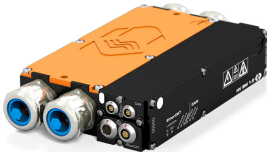
Fig. 3: HV Breakout Module 1.2 for measuring current, voltage and power in the separate HV+ and HV- lines between fuel cell stack and DC/DC converter.
