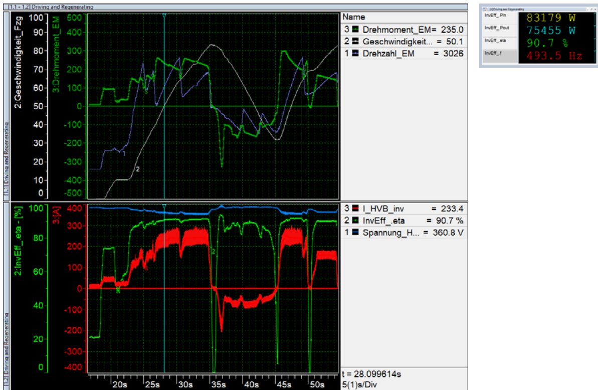
Fig. 5: Detail of a test drive of an electric vehicle with a nominal electric power of 75 kW and instrumented CSM Vector E-Mobility Measurement System (see Fig. 1). From the velocity profile shown in the upper plot (white), one can see when the vehicle accelerates and when it decelerates. Accordingly, the current shown in red in the lower plot is positive or negative. The vehicle's power electronics work as an inverter when driving, with efficiencies of over 90% at higher loads, and as a charger when the engine is operated as a generator during recuperation. When charging, efficiencies of up to 90% are also achieved. It can be seen that at small currents during load changes, the efficiencies of both the inverter and charger become worse. The calculation of the efficiencies can be done directly during the measurement or afterwards. It is done with the evaluation function (see Fig. 4) included in Vector's eMobility Analyzer function package (included in CANape, vMeasure exp and vSignalizer). This evaluation function also determines the frequency of the motor currents, the rotating field.
