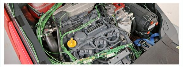
Fig. 3: The temperature and pressure sensors are installed in the specified locations in the engine compartment. The green cabling shows routing of the Type K thermocouple sensors to the measurement modules located outside the confined engine compartment.
