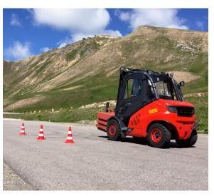
Fig. 1: In the high altitude test, a forklift truck is tested at 2,400 m in the Alps. After engine integration, the vehicle must function perfectly and still meets regulatory requirements.
