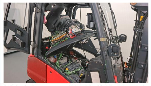
Fig. 5: This image shows the compact measurement modules in the cabin, located directly above the instrumented engine compartment.
