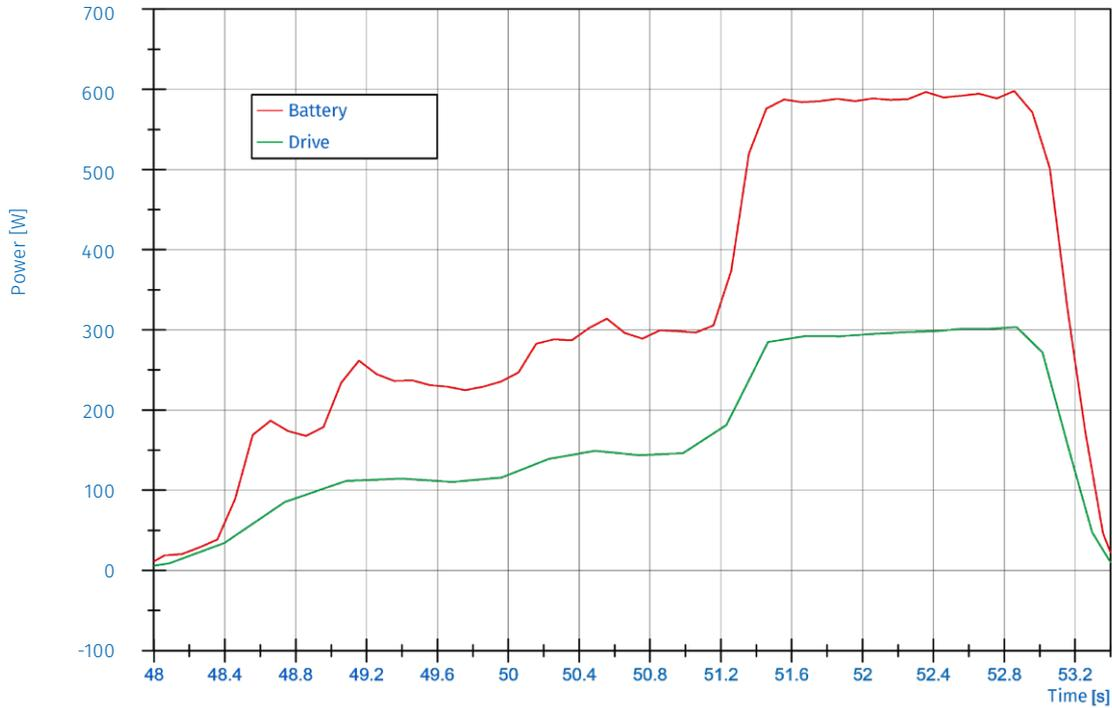
Fig. 5: Comparison of battery power and inverter power.
