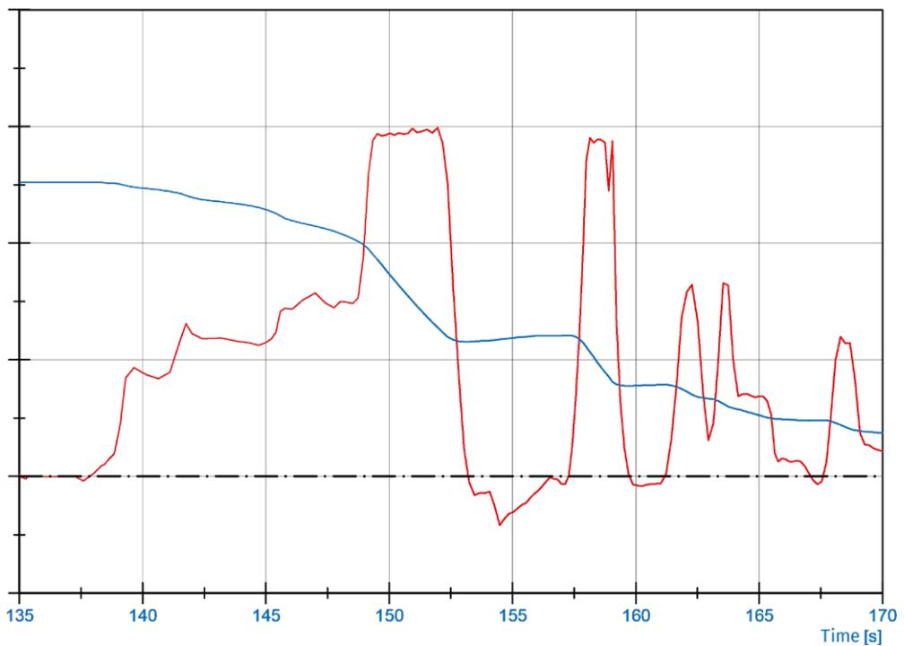
Fig. 6: The graph shows the battery charge level (blue) synchronously with the power delivery (red). While driving (power output > 0) the charge level steadily drops. During the braking process between 153 and 157 seconds, the charge goes up slightly – the effect of regeneration.
