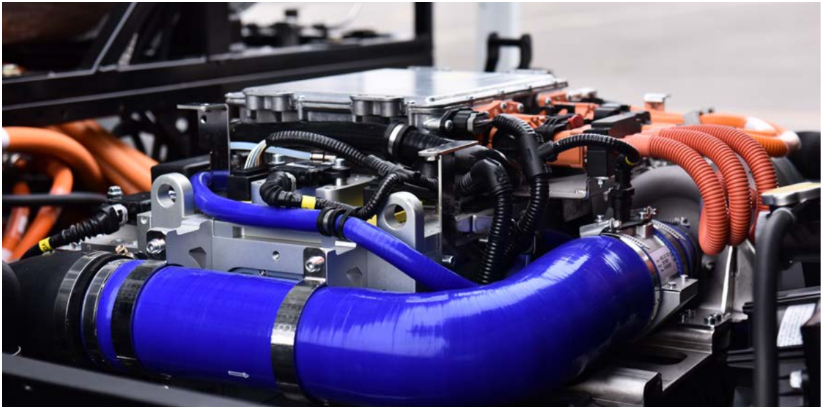
Fig. 2: The Bosch fuel cell system in the truck is fitted under the cab as standard. (Picture: Bosch, www.bosch-presse.de , ID #1e2e4630)
