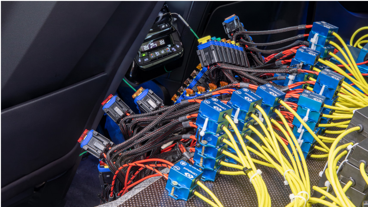
Fig. 1: Many measurement points, many measurement resistors: Some of the shunts were placed on the rear bench. (AVL List GmbH)
