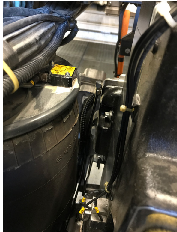
Fig. 4: Lasers are used to check whether collisions can occur between air bellows and the cast housing of the E-axle.
