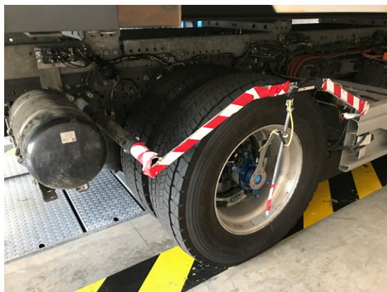
Fig. 6: RoadDyn measuring wheel on the E-axle for measuring the three-dimensional wheel forces ( F_x , F_y , F_z ) of \pm 180 kN and torques ( M_x , M_y , M_z ) of \pm 50 kNm.
