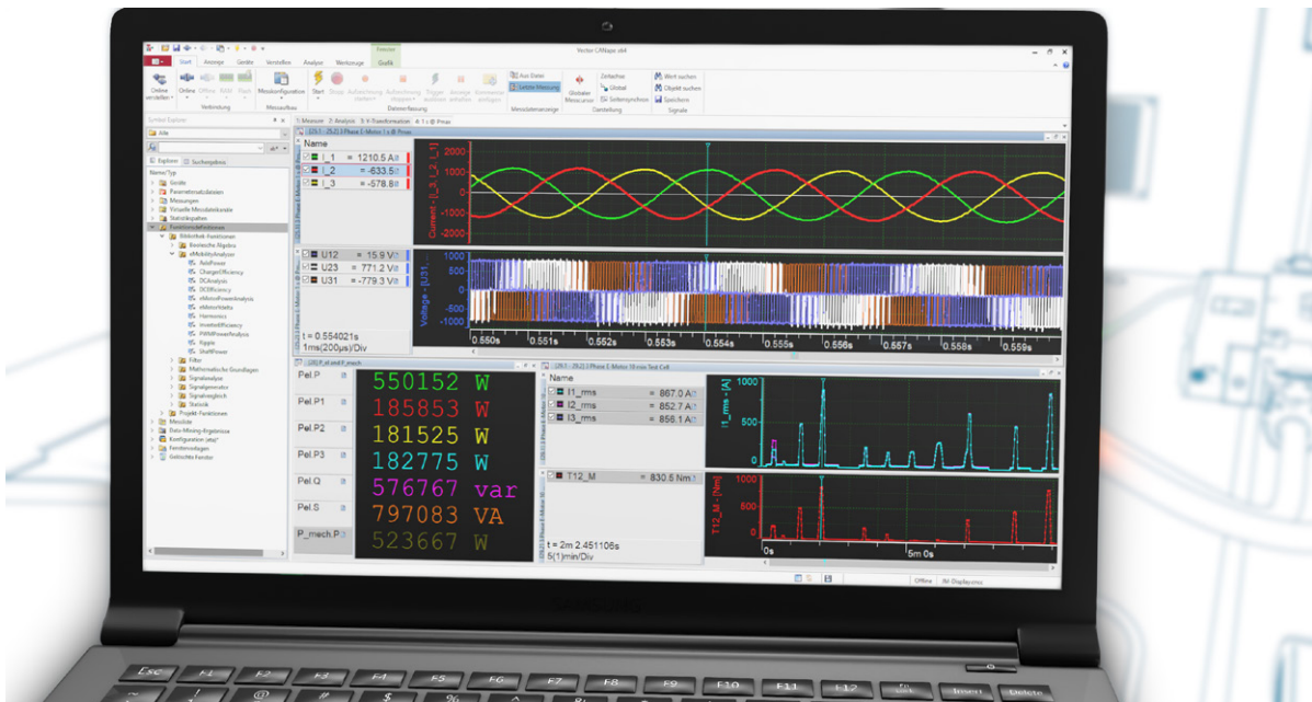
Fig. 5: Performance analysis of a ten-minute test run on the test bench with CANape. The raw values of the phase-to-phase voltages and string currents are shown in the upper area. The electrical values calculated in the process, such as active, reactive and apparent power, and the calculated mechanical power are listed numerically at the bottom left. The three calculated effective values of the motor currents are shown at the bottom right.
