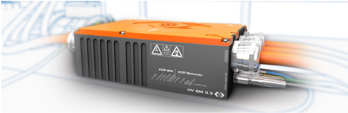
Fig. 7: HV Breakout Module 3.3.: The measurement system can be extended with further measurement modules via an EtherCAT and CAN interface. Via a Gbit Ethernet interface the data are sent to the measuring computer. Via the cable glands (shielded) HV cables up to 95 mm 2 are connected inside the housing.
