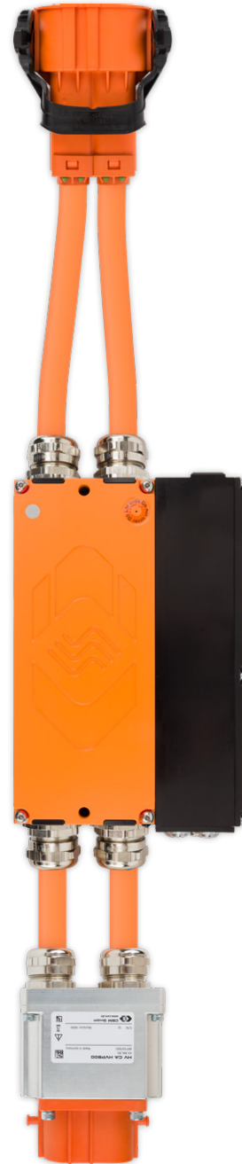
Fig. 4: CSM HV Breakout Module with connected cables, connectors and socket as a ready prepared, HV-safe plug-in system. The CSM HV BM system allows the distributed measurement and real-time analysis of high currents, voltages and outputs in the HV cables while driving at a sampling rate of up to 1MHz/signal.
