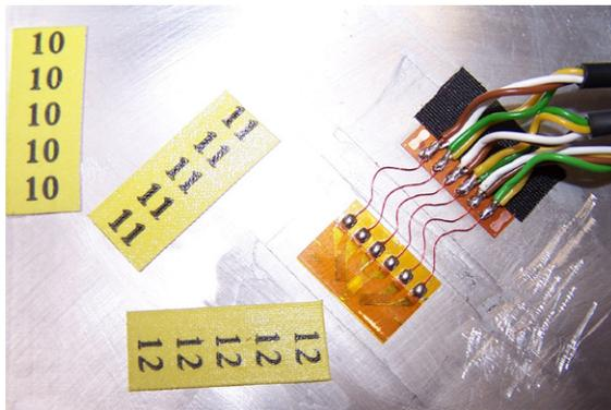
Fig. 2: Strain gauge as rosette on the outside of the battery housing
