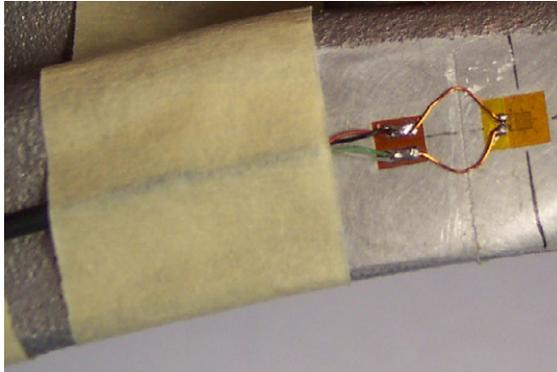
Fig. 1: Strain gauge on the outside of the housing
