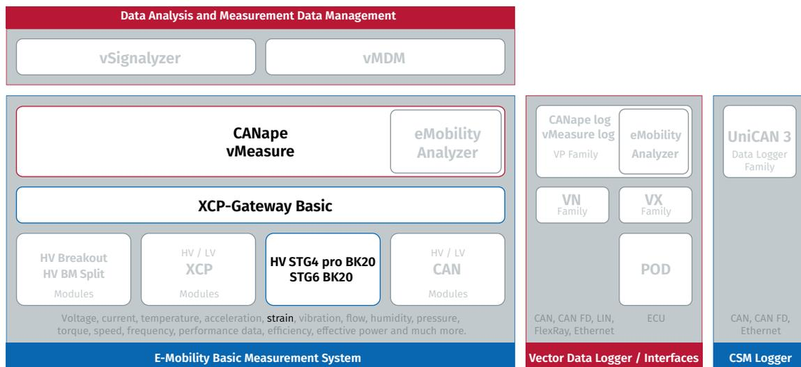
Fig. 3: The HV-safe strain measurement in HV batteries in the systematics of the Vector CSM E-Mobility Measurement System
