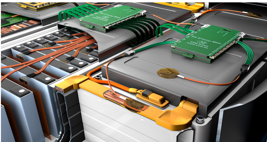
Fig. 3: HV DTemp IC single sensors on the module housing and busbar.
