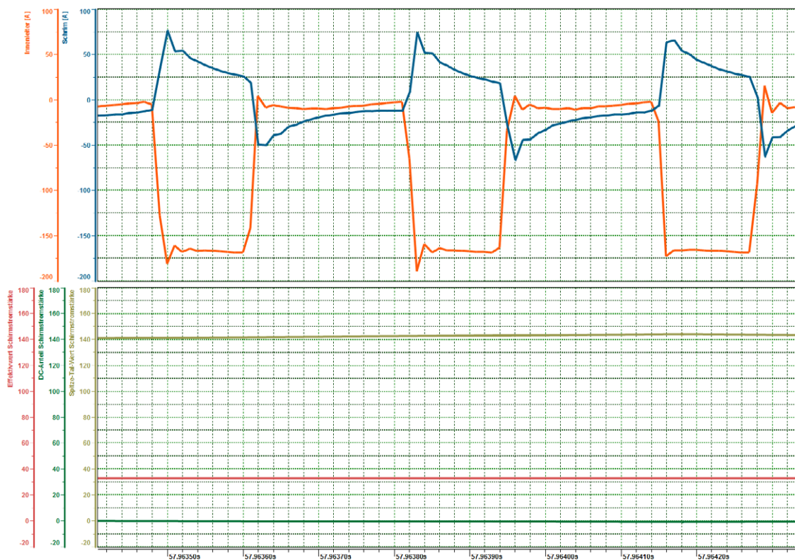
Fig. 4: Current on the inner conductor (orange) and on the shield (blue) as well as calculated signals of the eMobilityAnalyzer
