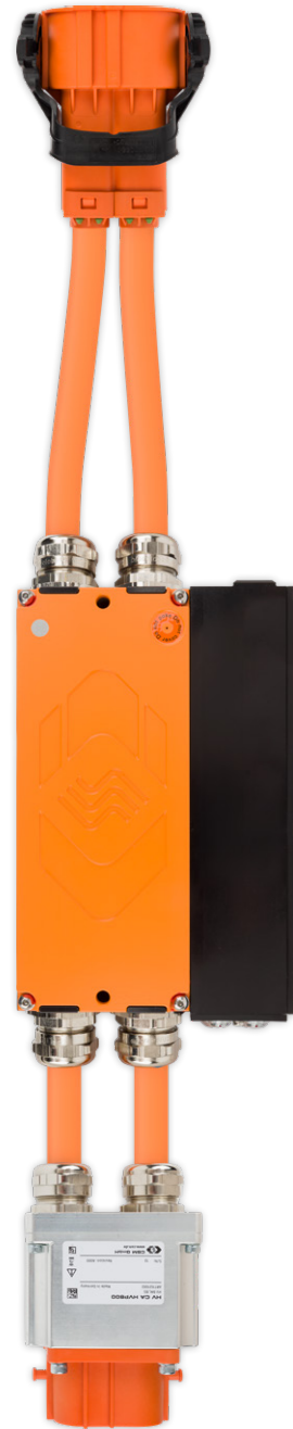
Fig. 4: CSM HV Breakout Module with connected cables, connectors and socket as a ready prepared, HV-safe plug-in system. The CSM HV BM system allows the distributed measurement and real-time analysis of high currents, voltages and outputs in the HV cables while driving at a sampling rate of up to 1MHz/signal.
