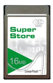
CSM PCMCIA Linear Flash Card Intel Series II+ compatible conforms to PCMCIA/JEIDA international standard and consists of multiple Intel's 28F008S5 (or 28F016S5) or compatible Flash memory devices and decoder IC mounted on a very thin printed circuit board using surface mounting technology.
