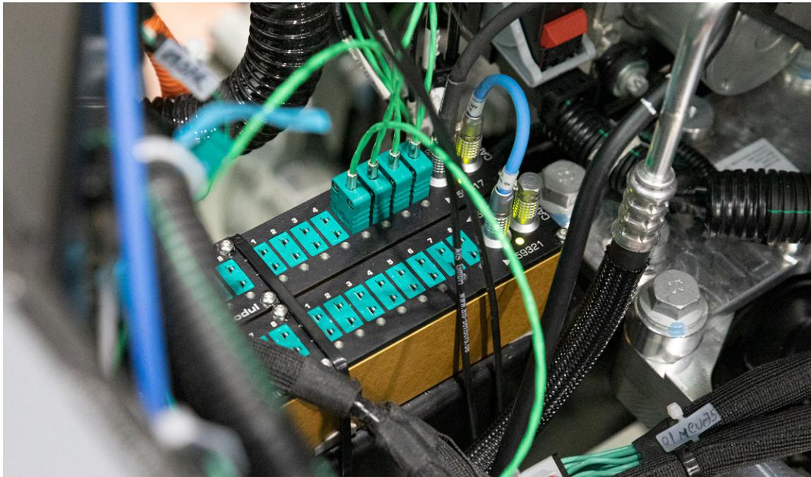
Fig. 2: In the vehicle compartment, but also on individual components, temperatures were acquired at 68 points via THMM pro thermal modules.
