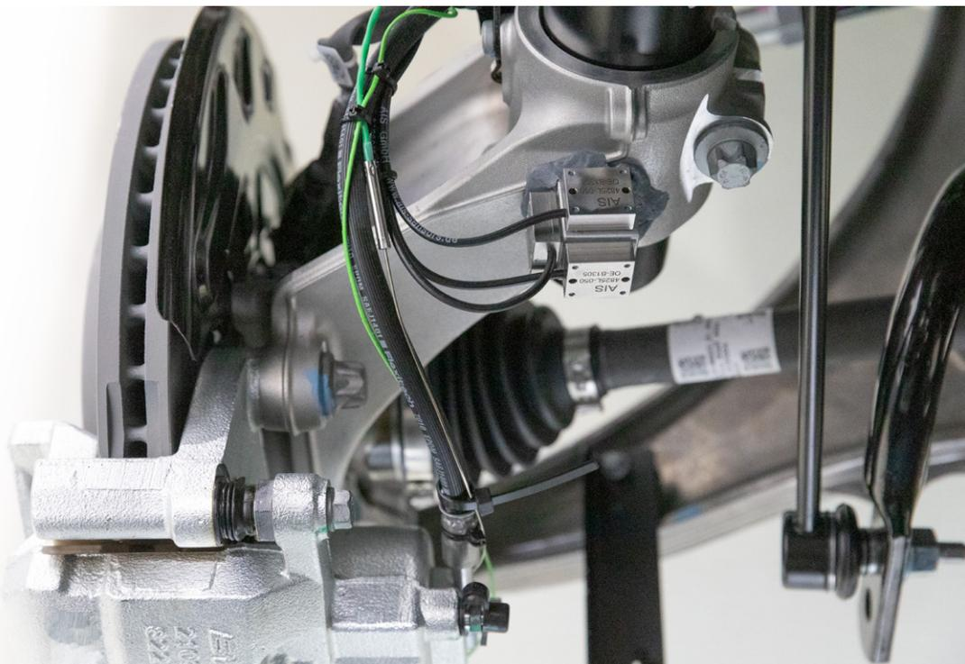
Fig. 3: Three uniaxial acceleration sensors record the movements of the wheel suspension in the x-, y-, and z-directions.
