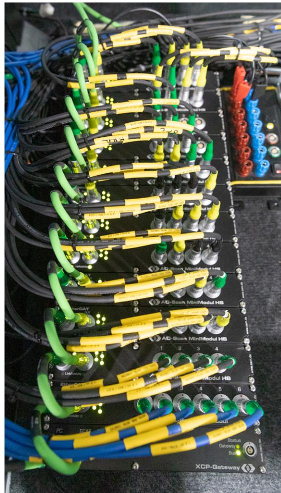
Fig. 4: Measurement data was transferred to an XCP-Gateway as an interface to the software via several STG6 ECAT and AD4 ECAT measurement modules.
