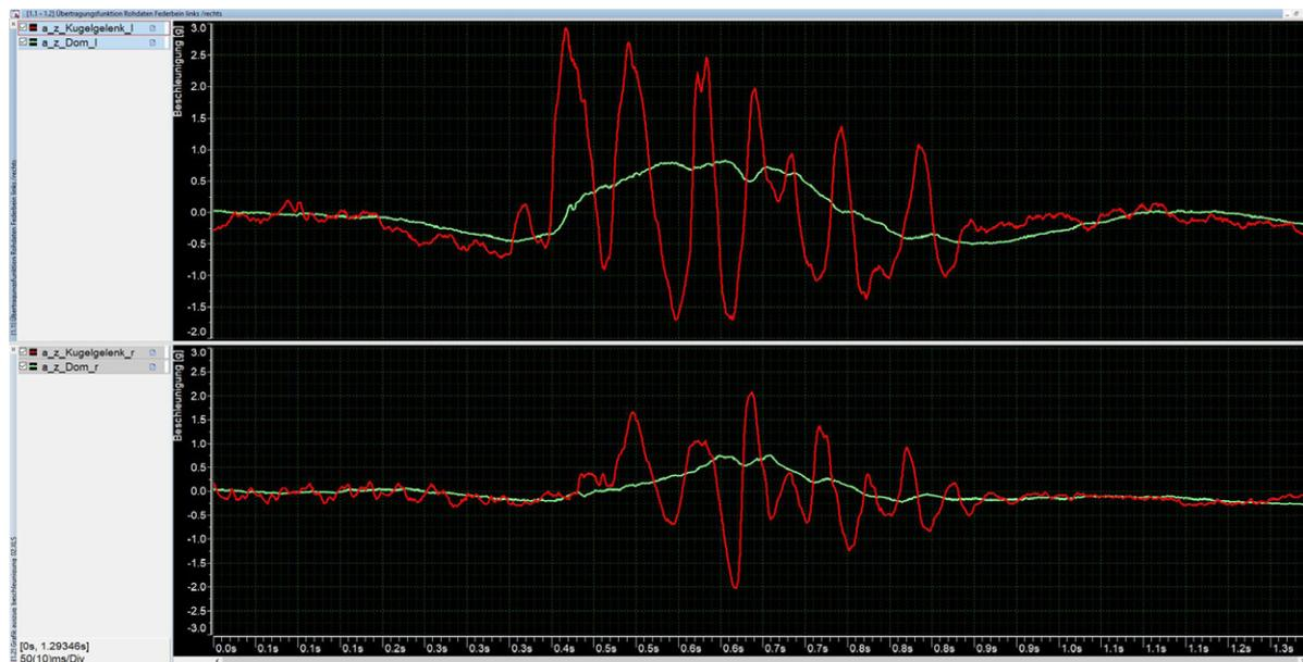
Fig. 5: Exemplary representation of the measurement data from acceleration sensors on the rear axle. The transmission factor from the spring-damper system (left and right) can be determined from the temporally correlated data.
