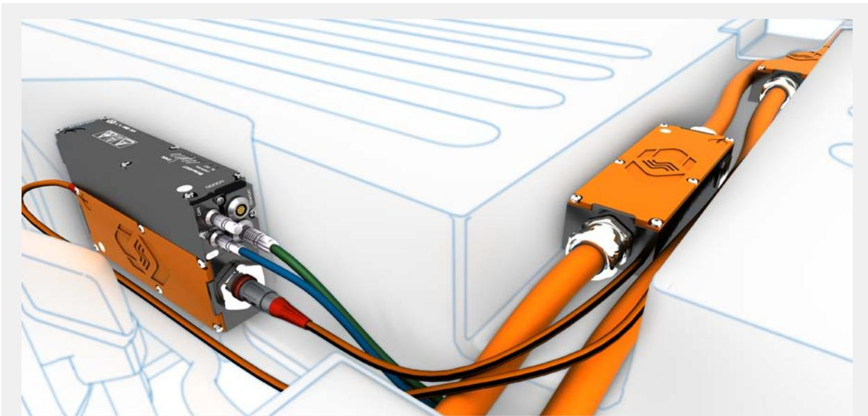
Fig. 4: High-voltage current and voltage measurement in a narrow cable duct. The Split Breakout Modules (HV SBM\_I, HV SBM\_U) for current and voltage are connected with high voltage safe sensor cables to the Split Acquisition Module (SAM). This is connected to the measuring computer via CAN or EtherCAT®.
