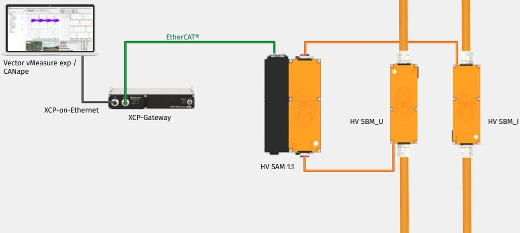
The current and voltage Split Breakout Modules are connected to the Split Acquisition Module via shielded high-voltage sensor cables using HV-safe
