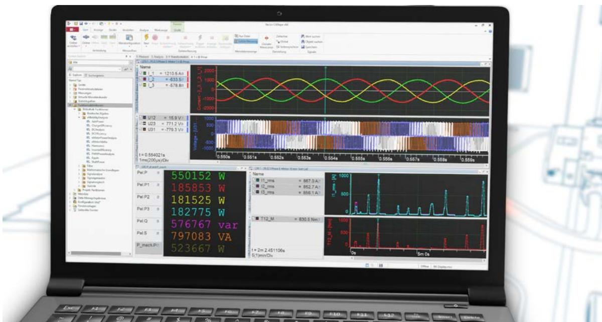
Fig. 4: Performance analysis of a ten-minute test run on the test bench with CANape. The raw values of the phase-to-phase voltages and string currents are shown in the upper area. The electrical values calculated in the process, such as active, reactive and apparent power, and the calculated mechanical power are listed numerically at the bottom left. The three calculated effective values of the motor currents are shown at the bottom right.
