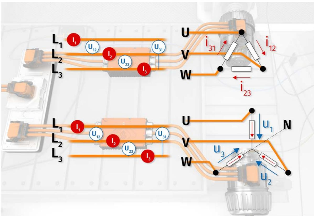
Fig. 5: Measurement circuit in the HV BM 3.3 for real-time power analysis with the Vector eMobilityAnalyzer. The star-triangle transformation is used to calculate the directly measurable conductor-to-conductor current strengths  $I_{12}, I_{23}, I_{31}$  and star voltages  $U_1, U_2$  and  $U_3$ .
