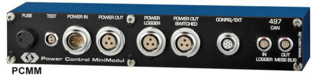
The Power Control MiniModule selectively switches on and off a data logger and measurement modules. The Power Control MiniModule can easily be configured for different application by use of the configuration plug. The power supply for a data logger and measurement modules is switched by KEY\_ON of the car (key on / off) or an external voltage. Alternatively, measurement modules and further external devices can also be switched using a signal supplied by the data logger.
